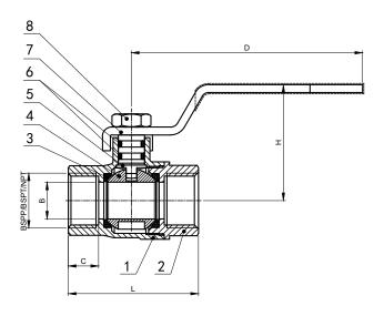
Suitable for use on Group 2 Gas and Group 2 Liquids as defined by Pressure Equipment Directive 2014/68/EU, and Pressure Equipment (Safety) Regulations 2016, as amended. Not suitable for use on Group 1 Gases or liquids.
