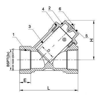
This valve is not suitable for use on Gases Group 1 & 2 or unstable fluids Group 1, as defined by the Pressure Equipment Directive 2014/68/EU.
